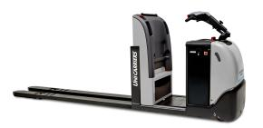
Efficient picking machine with highest performance. Lowlifting model with tiller arm or Ergo steering as option. AC powered, truck computer ATC and Friction Force for optimum drive wheel pressure.
