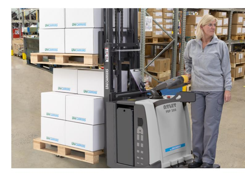
With a width less than that of a Euro-pallet, the PDP 200 has a total capacity of 2000 kg (1000 kg + 1000 kg in double pallet handling) and a maximum lifting height of 2090 mm. Its 2.2 kW AC-drive motor and driving speed of up to 12.5 km/h contribute to the unique pallet throughput of this efficient Double Stacker with ride on platforms (optional).
