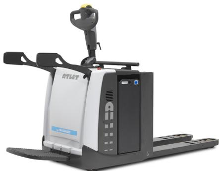
A high performance low lifter for cross docking or transport applications. Standard equipped with a durable casted fold-down driver platform, and ergonomic foldable side guards. Optional fixed driver protected platform and power steering makes this low lifter the perfect partner in extended work cycles and multi shift operations.
